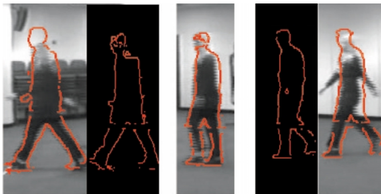
Figure 7. Cropped, sample frames from a tracked test sequence. The same learned model and test sequence is used as in Fig. 6, but now the test sequence is periodically blanked out, to test robustness to occlusion (see also video walk3occ.mpg ).
